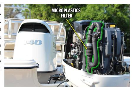
Previewed to the world's boating industry in Fall 2020 as the first micro-plastics collection device designed for installation on outboard motors, Suzuki has continued to test and refine this product, which has the power to make Suzuki owners part of the solution to the global challenge of micro-plastics pollution. Filter systems have arrived in the United States and are currently being tested on vessels stationed at the new Suzuki Marine USA Technical Center in Panama City, Florida.
