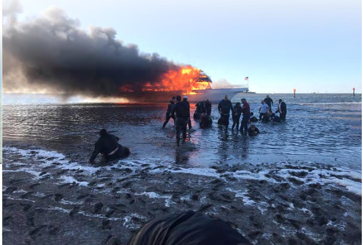
During the voyage, the captain received the high-temperature alarm for the port engine's jacket-water system. He did not shut down the engine but instead left it idling. Doing so allowed the overheating engine to continue to generate excessive heat, which in turn affected the exhaust tubes and ignited their surrounding structures. The vessel owner had not provided specific guidance to its vessel captains about how to respond to high-temperature alarms.
