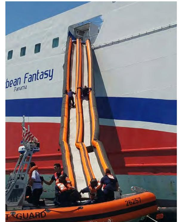
Figure 60. *Caribbean Fantasy*’s marine evacuation system deployed on the starboard side. PHOTO BY COAST GUARD
