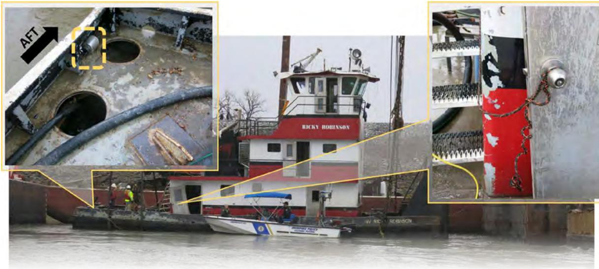
**Figure 41. *Ricky Robinson* post-salvage. Two inset photos show (at left) both aft voids missing hatch covers, with a yellow square highlighting where the submersible pump was found, and (at right) the open starboard engine room door that was tied off to the stairs.**
