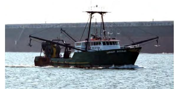
**Figure 37. *Langley Douglas* with its outriggers extended and paravanes stowed at the end of the outriggers.**
