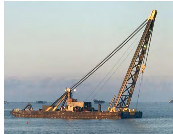
**Figure 47. *Troy McKinney*, with the A-frame boom mounted on the barge's stern.**
