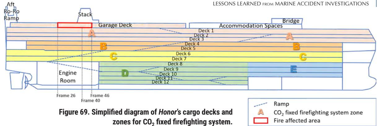
**Figure 69. Simplified diagram of *Honor's* cargo decks and zones for CO<sub>2</sub> fixed firefighting system.**
