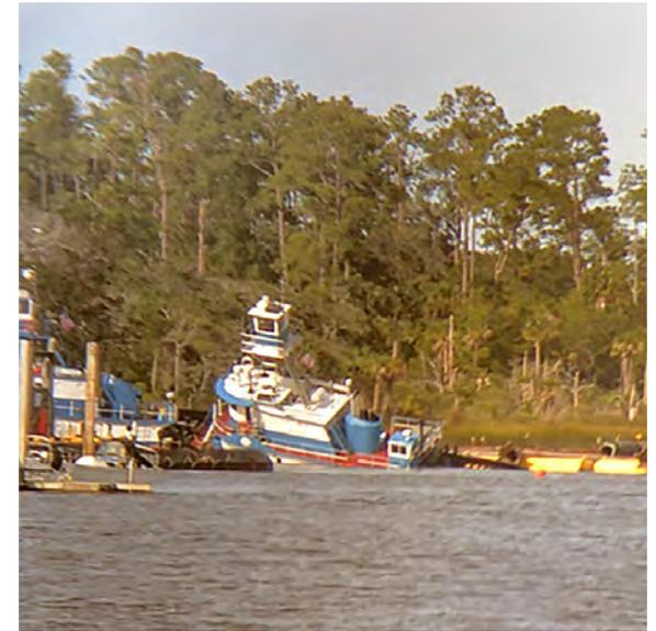
**Figure 83. *Atlantic Raider* aground on the shallows of the west side of the Blount Island Channel. Note that the port quarter is under water up to the lower wheelhouse deck.**
