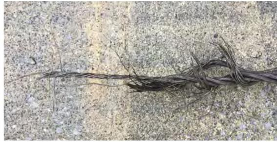
**Figure 19. Strands on wire rigging that was recovered by investigators indicated that the wires had fractured while in tension.**
