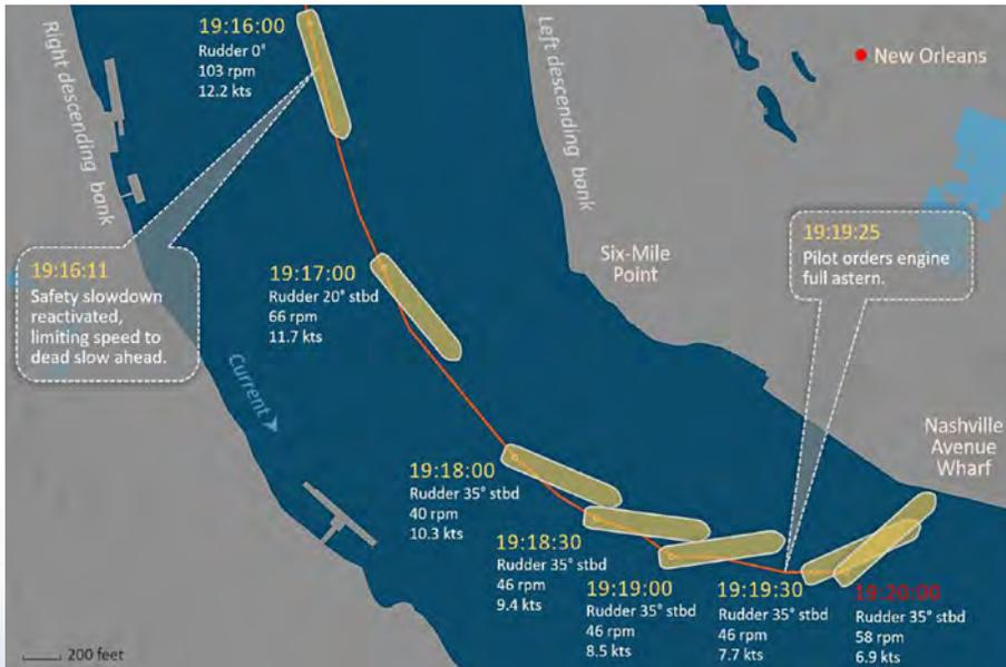
**Figure 25. Trackline of the *Mia S* over the last 4 minutes leading up to the accident shows changes in the vessel's heading and speed over ground following an engine slowdown.**
