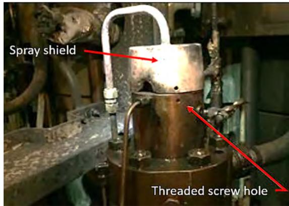
**Figure 49. Inboard view of the no. 6 cylinder fuel pump and top cover postaccident, with the spray shield slightly elevated to illustrate alignment of fastener holes.**
