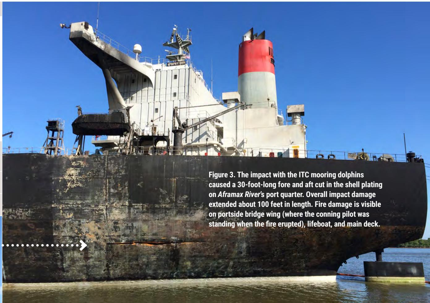
Figure 3. The impact with the ITC mooring dolphins caused a 30-foot-long fore and aft cut in the shell plating on *Aframax River*'s port quarter. Overall impact damage extended about 100 feet in length. Fire damage is visible on portside bridge wing (where the conning pilot was standing when the fire erupted), lifeboat, and main deck.
