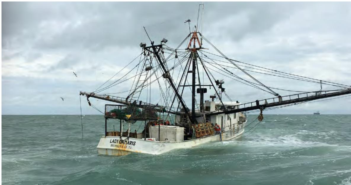
The NTSB determined that the probable cause of the flooding and sinking of the fishing vessel *Lady Damaris* was the captain's decision to continue to operate with a known hull leak.
