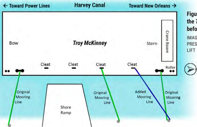
**Figure 46. Mooring line arrangement for the *Troy McKinney* on June 1 (six days before the accident).**
