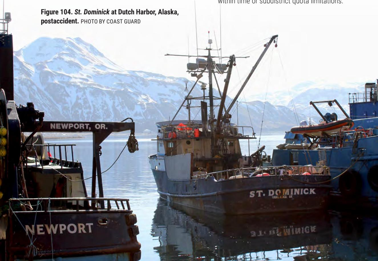
On March 6, 2017, about 0009, the uninspected commercial fishing vessel *St. Dominick* grounded in Pumicestone Bay, Alaska. The engine room flooded within 10–20 minutes of the grounding, and the four crewmembers abandoned the vessel a short time later. None of them were injured, and no pollution was reported. The vessel, valued at \$1.1 million, was deemed a constructive total loss.
