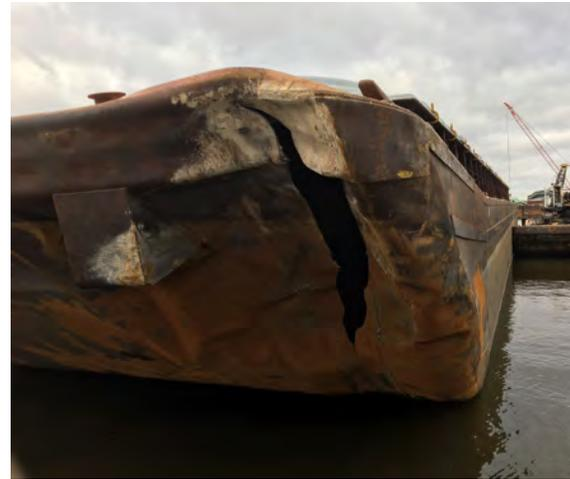
**Figures 11 and 12. Damage from allision: (above) raked bow of port lead barge, ART 35157; (below) downstream view of the swing bridge's fixed pier near the left descending bank that was struck by the barge.**
