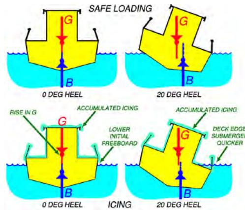
**Figure 32. A diagram from the Coast Guard's guide on vessel stability illustrates the negative effect of icing.**
