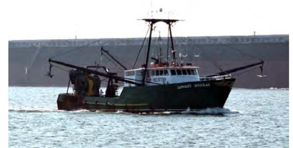
**Figure 37. *Langley Douglas* with its outriggers extended and paravanes stowed at the end of the outriggers.**
