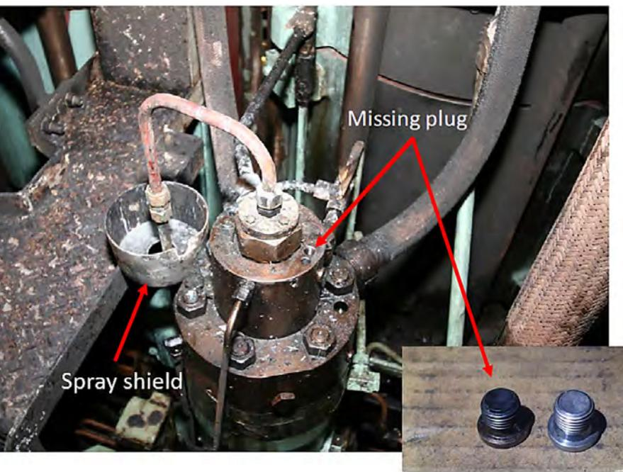
**Figure 50. Fuel pump housing and top cover for the no. 6 cylinder, with missing pipe plug. The lower-right image shows the dislodged pipe plug (left) next to a new unused plug.**
