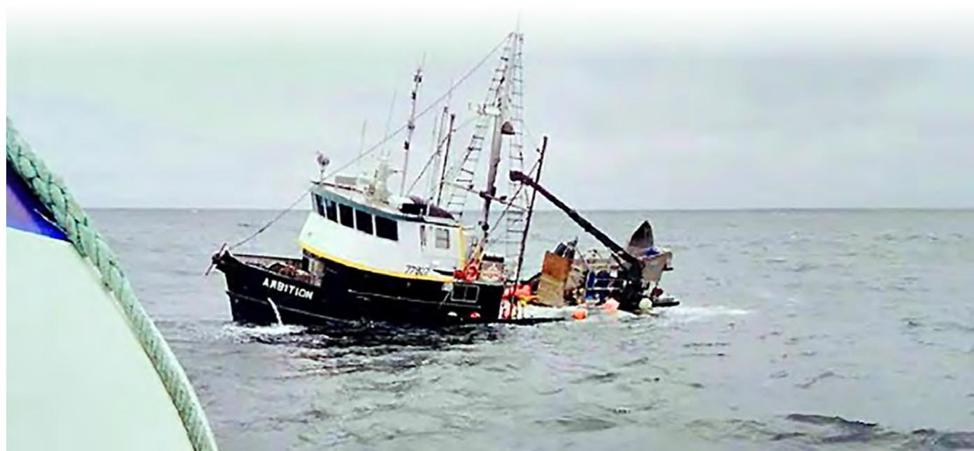
securely dogged. The captain said that when they opened the hatch, there was more water in the space than they could pump out. The captain and the engineer closed and dogged the hatch and proceeded back to the wheelhouse.
