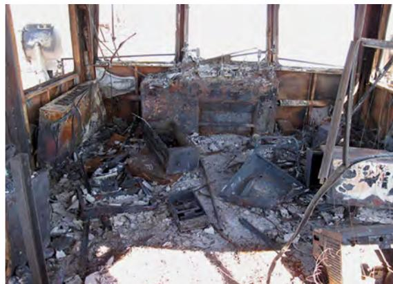
Figure 66. Charred remains of the wheelhouse.
