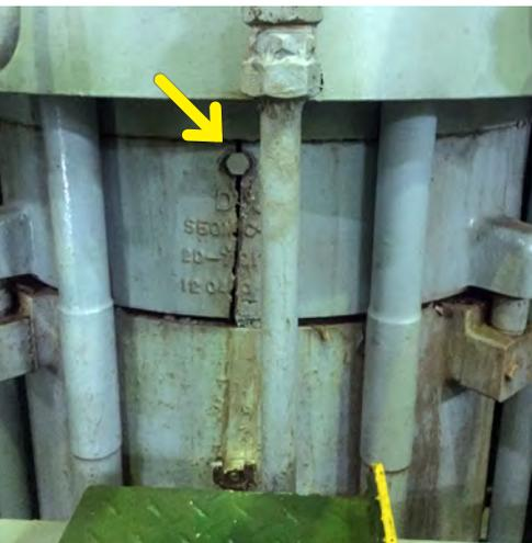
**Figure 100.** Cracked cooling jacket on main engine no. 3 cylinder, postaccident. Arrow identifies one of four hex head securing bolts for the jacket cover.
