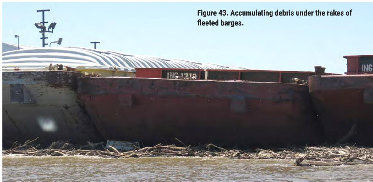
Figure 43. Accumulating debris under the rakes of fleeted barges.
