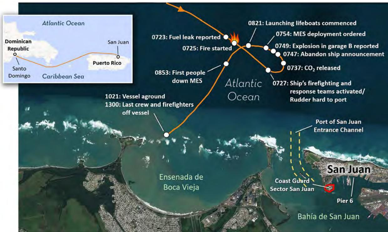
Figure 59. Automatic identification system (AIS) track of the *Caribbean Fantasy* and timeline of events.
