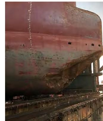
**Figure 101.** Damage to *Nenita's* bulbous bow, starboard side.
